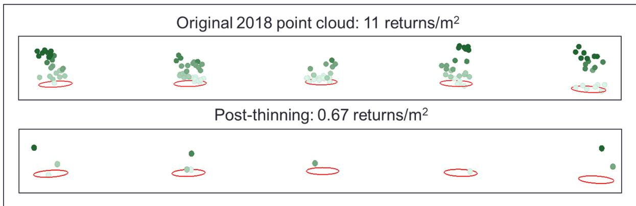
Figure 4: 2018 LiDAR HAG metrics extracted for same transect as Fig. 3, before and after thinning
